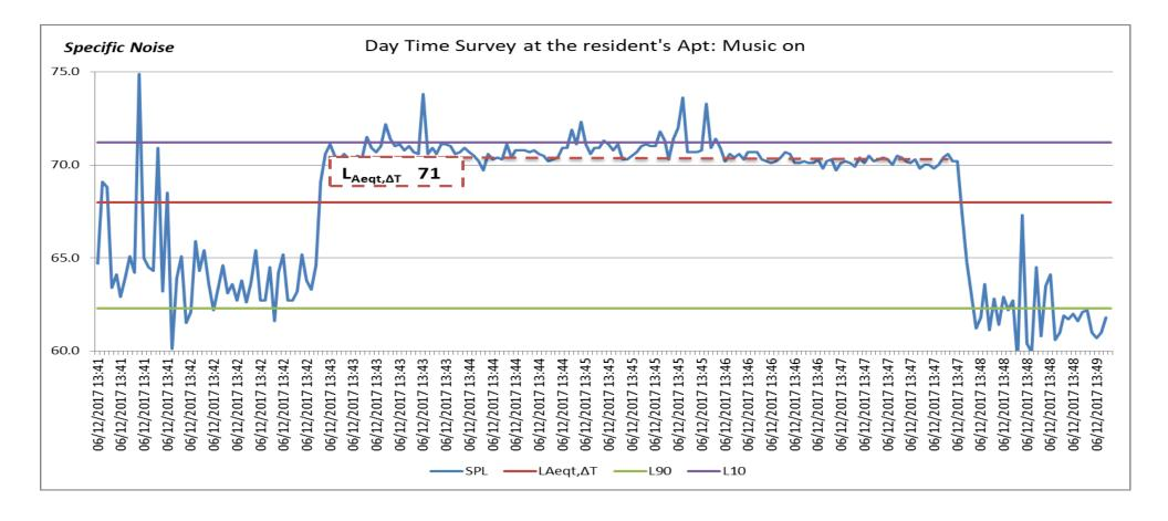
The lead and lag one minute monitored in the graph, specify the residual noise level; hence the true  $L_{Aeq,t}$  is 71 dB(A) Therefore, the difference between Specific & Residual Noise is 71 – 59 = 11 dB (A)
