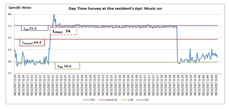
The specific noise level is the continuous A-weighted sound pressure level at the assessment position over a given reference time interval that is produced by the noise source that is being investigated for assessing the likelihood of complaints.
