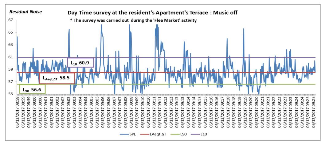
The residual noise level is the continuous A-weighted sound pressure level when the specific noise source is suppressed to a degree that it does not contribute to the background noise.
