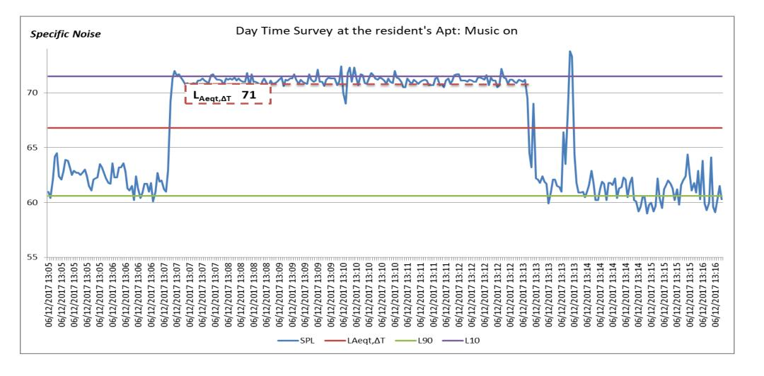
The lead and lag two minutes monitored in the graph, specify the residual noise level; hence the true  $L_{Aeq,t}$  is 71 dB(A) Therefore, the difference between Specific & Residual Noise is 71 – 59 = 12 dB (A)
